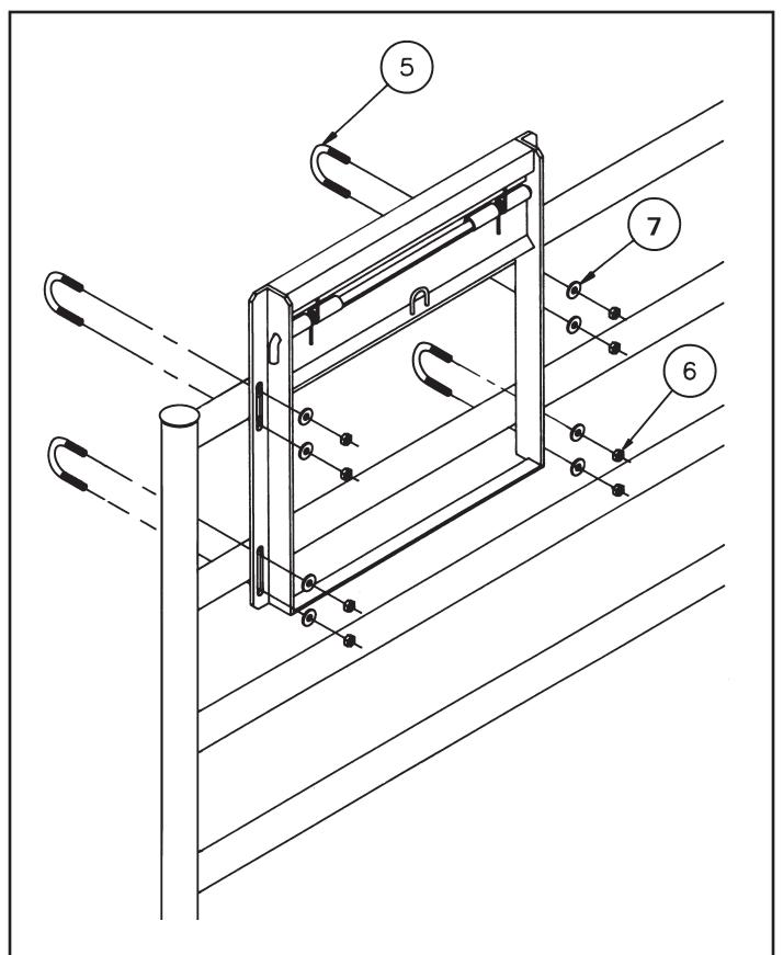
This view shows the assembly of the Portable Care Center's latch. Note the position of the torsion springs. The spring extension legs should be facing outward.
